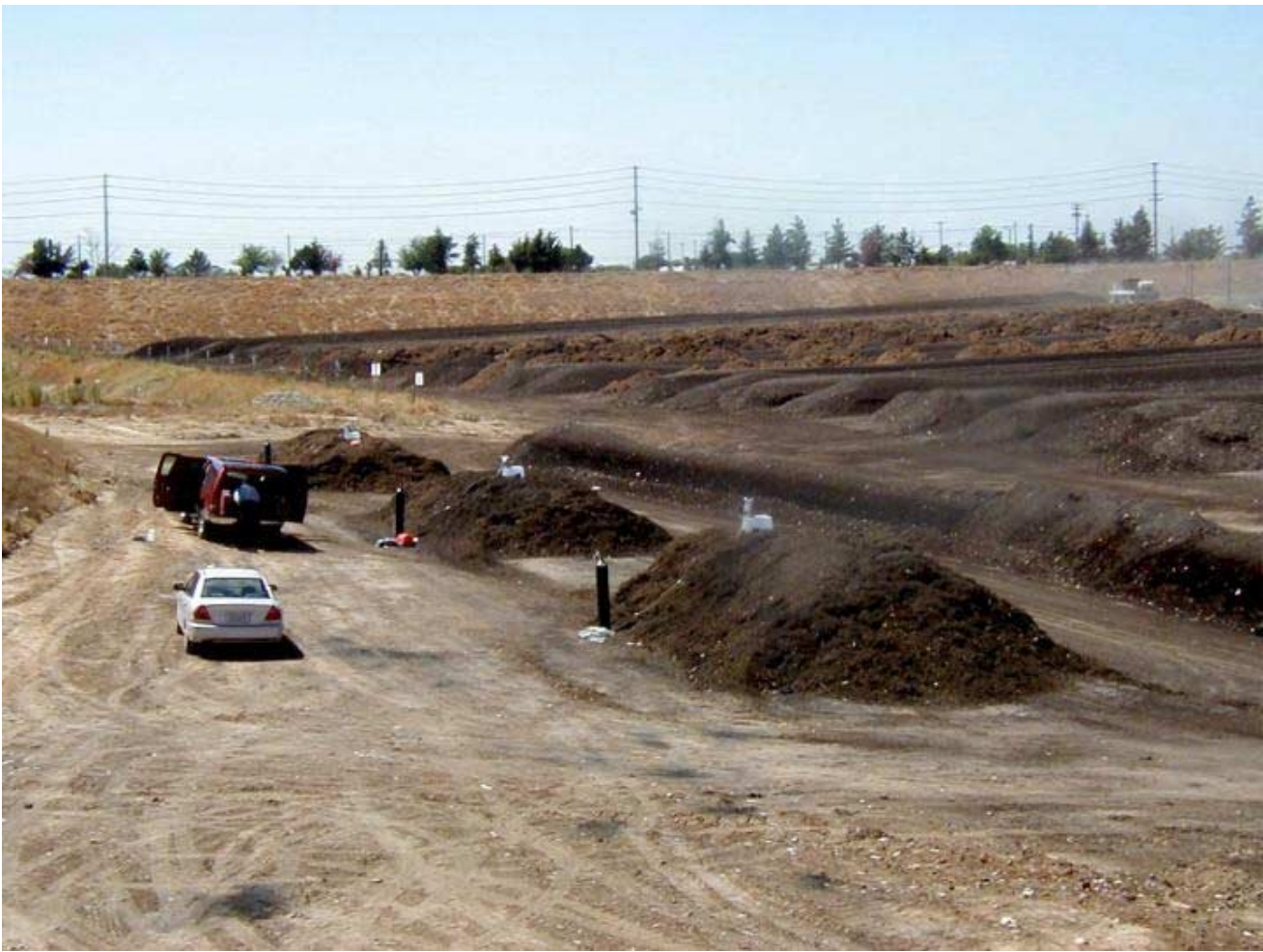
Photograph 2: Three pilot study compost piles with flux chambers during sampling. The pile in the front contained 25 percent wood ash, the middle pile contained 12.5 percent wood ash, and the farthest pile contained no wood ash.
